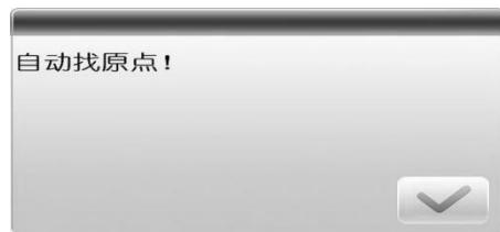
5. The X-axis drive slider moves to the left, while the Y drive slider moves backward; they stop when reaching their origins.
